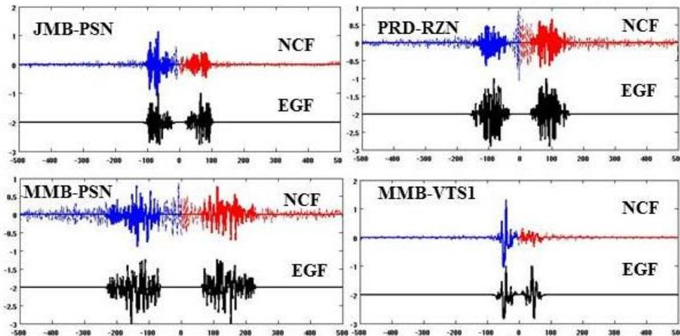
Fig. 2. NCFs and EGFs for station pairs JMB-PSN, PRD-RZN, MMB-PSN and MMB-VTS1 (blue lines). Red lines denoted the correlated signals from reverse pairs
