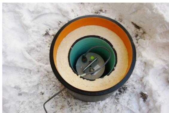
Fig.2. Seismometer CMG40T and thermo isolation
