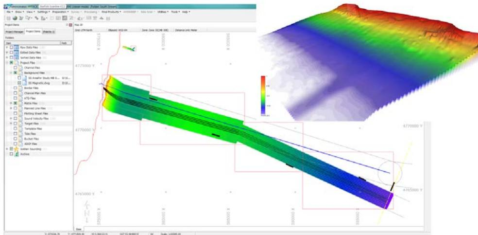
**Figure 1. Pasha dere – Varna.** Digital terrain model of a part of the nearshore area based on MB data.
