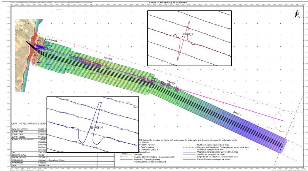
**Figure 4. Pasha dere – Varna.** Magnetic anomalies registered as a result of a magnetometer/gradiometer survey
